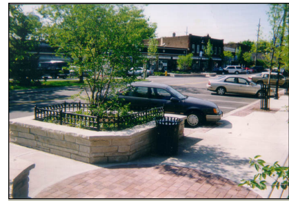
In addition to providing ease of access for motorists, the angled parking format can typically accommodate more parking spaces than the parallel parking format.
