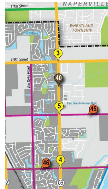
Figure 5.3 Capacity Improvements (such as Right turn lanes) are needed at the major intersections with IL 59
