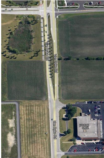
Figure 4.8 Shared Use Path Gap The adjacent picture shows one such location along Van Dyke Road where a shared-use path on the west side of the road abruptly ends.
