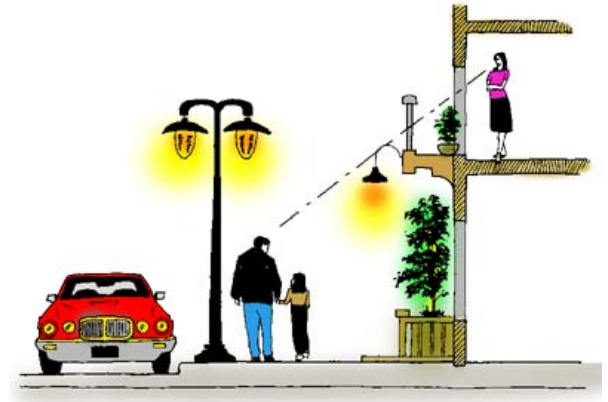
Pedestrian safety enhancements include on-street parking (acts as buffer, and slows cars down) and street lighting (buffer). Amenities include the decorative lighting and street plantings.
