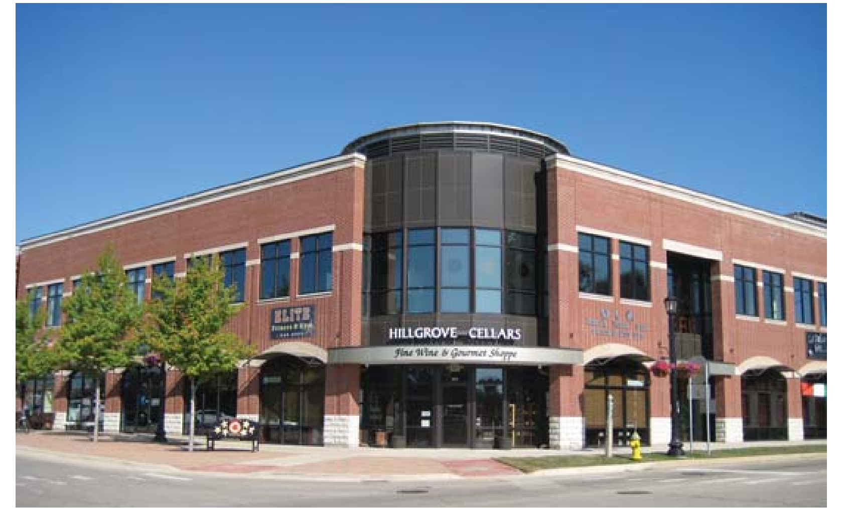
Defined entrance and use of metal materials at corner helps to diversify building materials while adding visual interest. Note: Arched metal awnings above windows on first floor.
