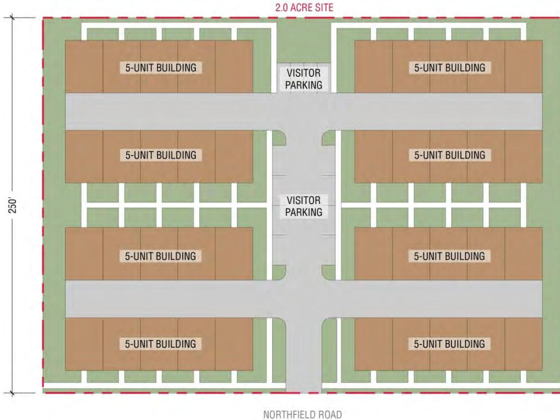
The lower density alternatives could be created in the same layout, but with only three or four units in each building (and larger average unit sizes).
