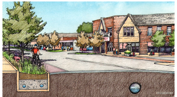
Tree planters with stormwater filtration
