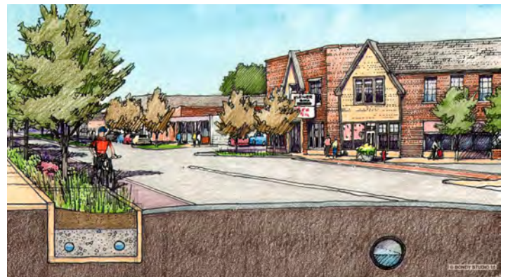
Tree planters with stormwater filtration
